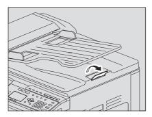
· To prevent misfeeding, do not leave originals or turn OFF/ON the equipment with originals on the Reversing Automatic Document Feeder.
