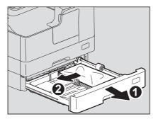
Check that the guide width is correct, there is no folded/curled paper or overloading, and then close the drawer.
