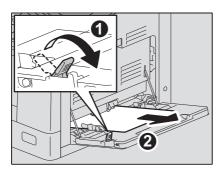
2 Check beneath the transport guide inside of the side cover. Check if any paper is misfed under the transport guide behind the transfer unit. P.206 "Paper misfeeds inside of the side cover"
